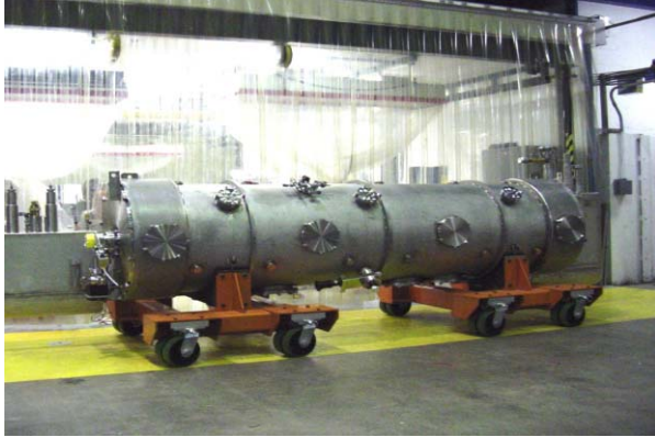
Figure 7: Three cavities per cryomodule prototype (medium \beta structure of the sc linac) constructed at JLab.
