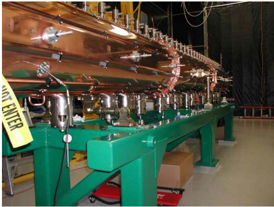
Figure 3: Picture alongside assembled DTL tank 3 with drift tubes and post couplers installed at LANL ready for shipment to Oak Ridge.
