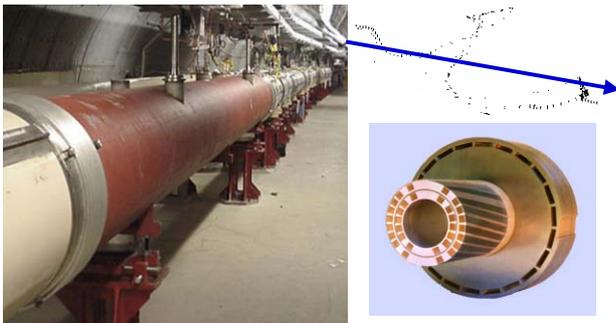
Figure 7. Siberian snakes, the spin trajectory inside and the end windings of the helical dipoles.
