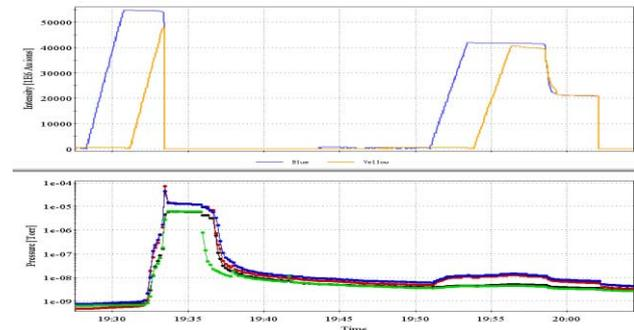
Figure 5 – Vacuum breakdown induced a beam abort during filling of the second ring with 110 bunches.
