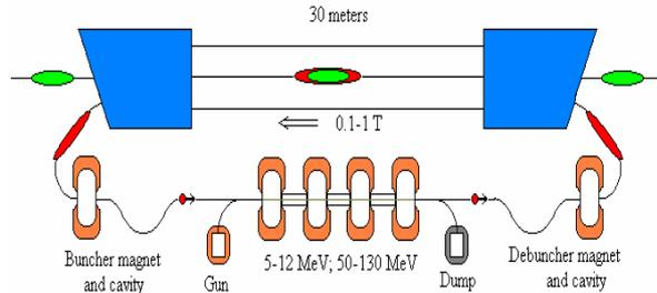
Figure 11. Schematics of the proposed electron cooling system based on an energy recovering linac.
