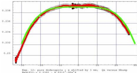
Figure 9. Measured dodecapole effect: tune shift (left) as a function of bump amplitude (right).
