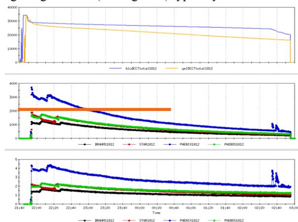
Figure 2. Au store: beam current ( $\times 10^6$  ions), collision rates (Hz) compared to design (horizontal line), specific luminosity ( $\text{Hz}/10^{18}$ ) (expected: 5 for Phenix, 2.5 others)
