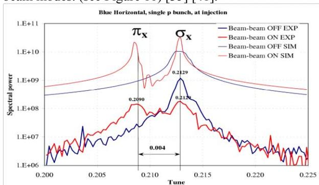
Figure 10. Coherent beam-beam modes in RHIC.
