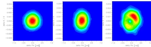
Figure 4. Tomographic reconstruction of bunch density before, at and after instability (10 msec growth rate)[19]
