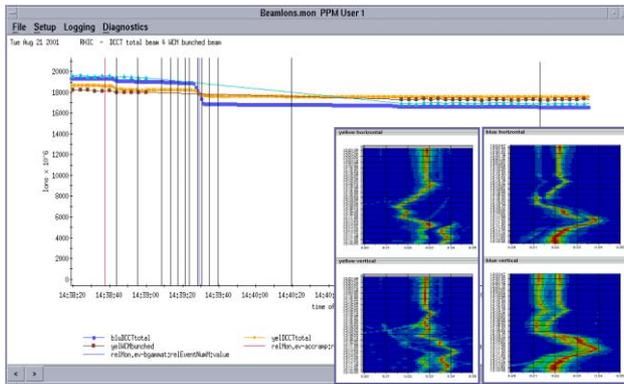
Figure 3. A RHIC ramp (DCCT beam intensity) and tune measurements on the ramp [14].
