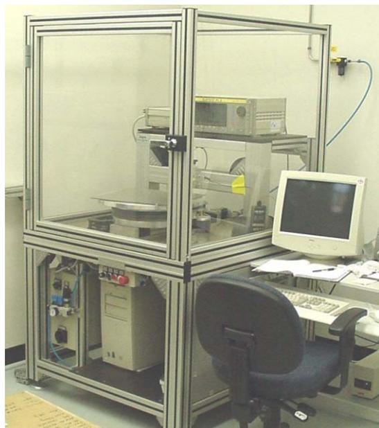
Figure 6: Eddy Current Scanning system used at Jlab for defect scanning of the niobium used for SNS cavities.
