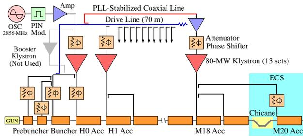
Figure 1: Diagram of improved RF.
