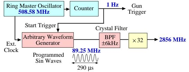
Figure 2: Block diagram of RF reference generator.
