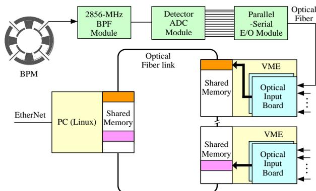
Figure 4: Block diagram of BPM data acquisition system.
