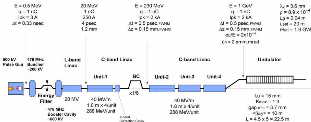
Fig.2 SCSS beam line layout at final stage (beam energy 1 GeV, radiation wavelength 4 nm).
