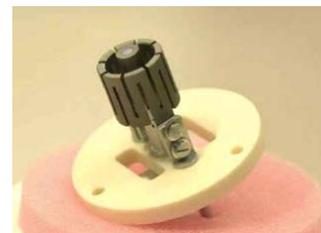
Fig.3. CeB<sub>6</sub> single crystal cathode with graphite heter.
