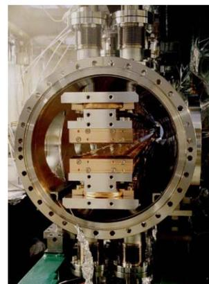
Fig.4 The 37 m in-vacuum undulator installed in the 8 GeV storage ring at SPring-8 in 2001. We use same design for SCSS project.
