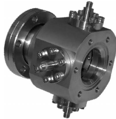
Figure 4: Design of a \lambda/4 stripline beam-position monitor.
