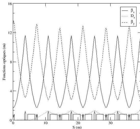
Figure 1 : Optical functions
