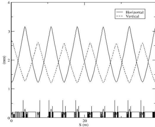
Figure 2 : rms C.O. distortion
