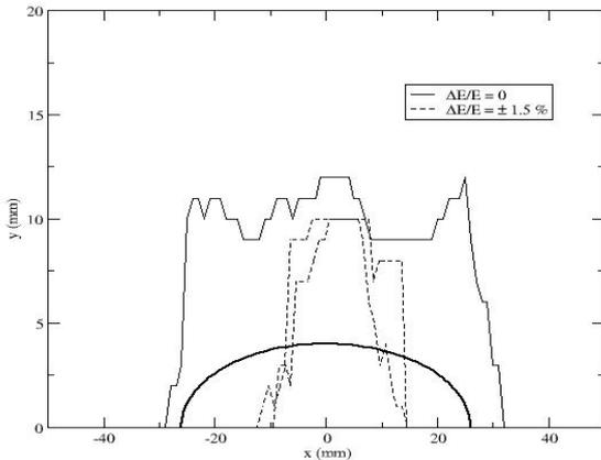
Figure 5 : Dynamic aperture at injection including Eddy current and multipole effects
