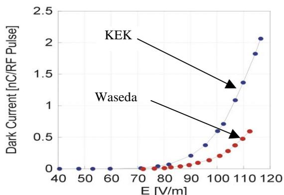
Fig. 1 Dark current measured under the beam test with the high gradient acceleration fields
