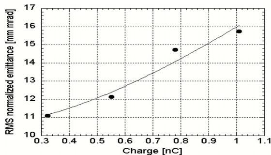
Fig. 3 Beam emittance measured by slit scan method as the function of bunch charge
