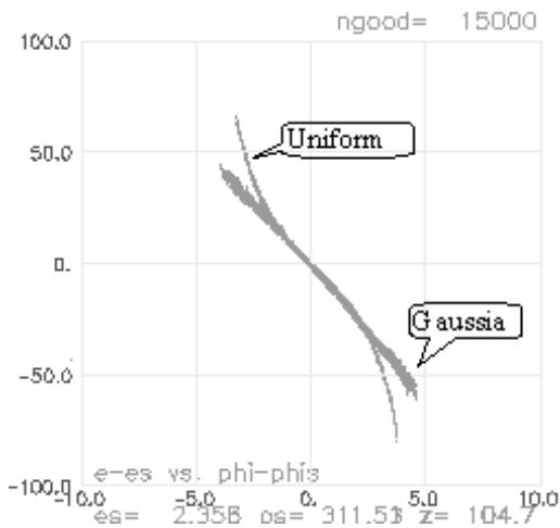
Figure 3: photoelectron beam longitudinal phase space distribution for uniform and Gaussian lasers.
