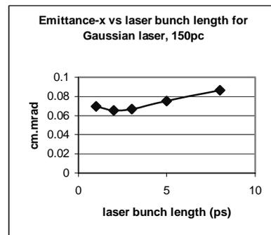
Figure 5: transverse emittance as a function of laser pulse length.
