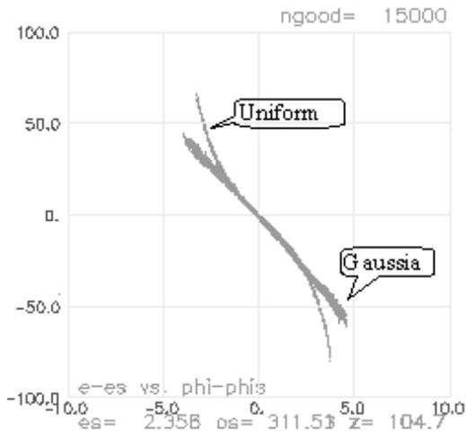
Figure 3: photoelectron beam longitudinal phase space distribution for uniform and Gaussian lasers.
