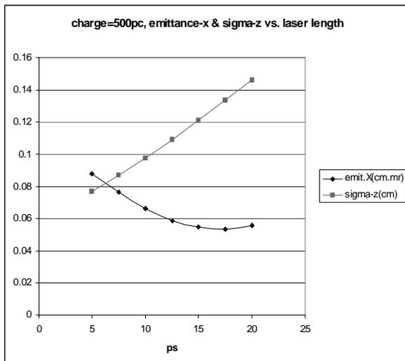
Figure 7: transverse emittance and bunch length as a function of the laser pulse length for a 0.5 nC charge.
