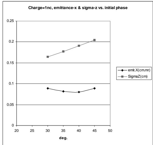
Figure 8: the transverse emittance and bunch length as a function of the RF gun phase for a 1.0 nC charge
