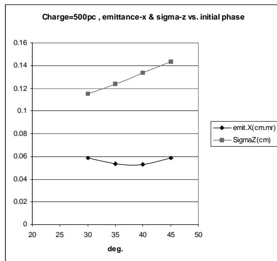
Figure 6: the transverse emittance and bunch length as a function of the RF gun phase for a 0.5 nC charge.
