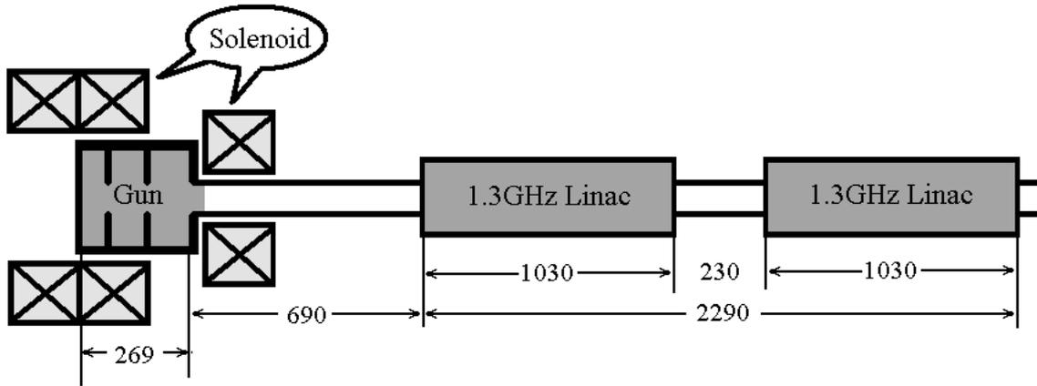
Figure 2: The schematic set-up of L-band Photoinjector.
