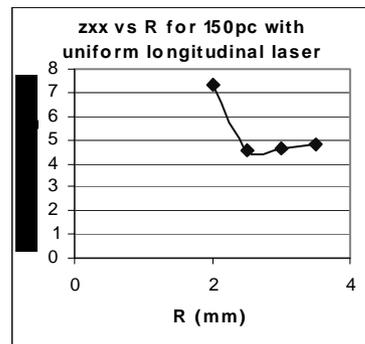
Figure 4: 6-D emittance optimization for laser spot.
