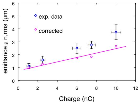
Fig. 4 : Transverse normalized emittance at the linac exit, vs. bunch charge, with and without the space charge correction. The drive laser pulse width is about 60 ps.
