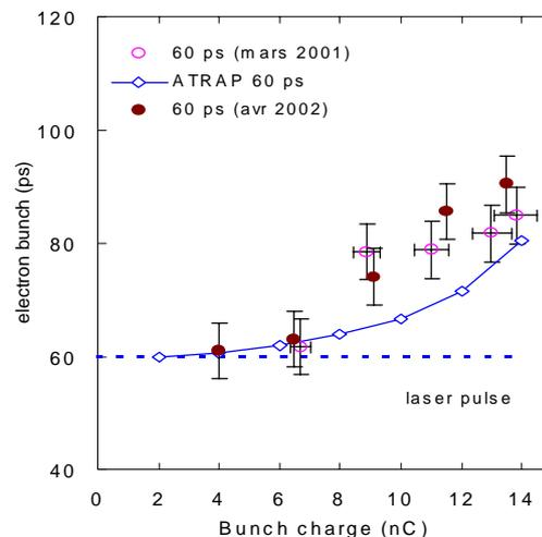
Fig. 2 : Length of the electron bunch at the linac exit, as a function of the bunch charge (laser spot diameter on photocathode = 4 mm).
