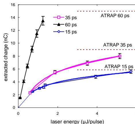
Fig. 3 : Bunch charge measured at the linac exit as a function of the drive laser pulse energy. The slope at the origin corresponds to the cathode quantum efficiency : 1.0 % for the 15 and 35 ps data and 3% for the 60 ps data.
