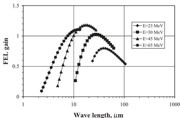
Figure 4: FEL gain for different energies of the driving electron beam as calculated with the code [5].
