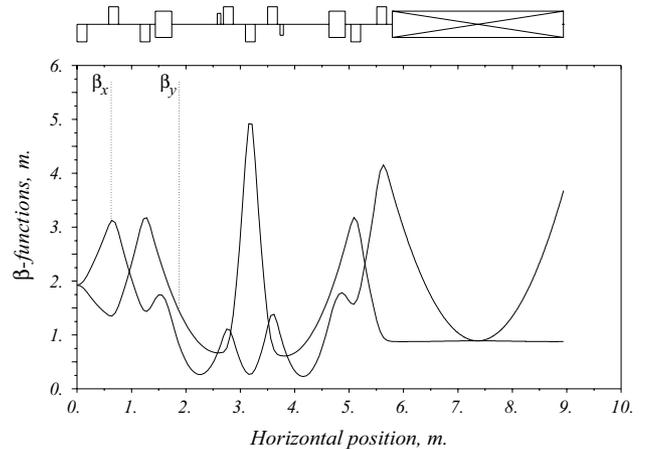
Figure 3: Optical functions in the undulator and in the S-bend as calculated with the MAD code at an energy of 45 MeV and an undulator strength  $K_{rms}=1.0$ .
