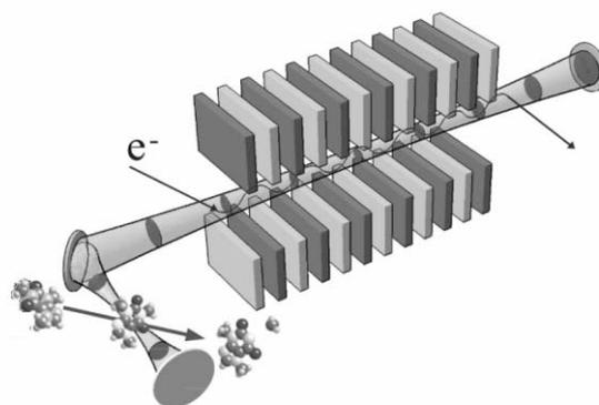
Figure 5: The L-shaped optical resonator and a typical layout of an intra-cavity experiment.
