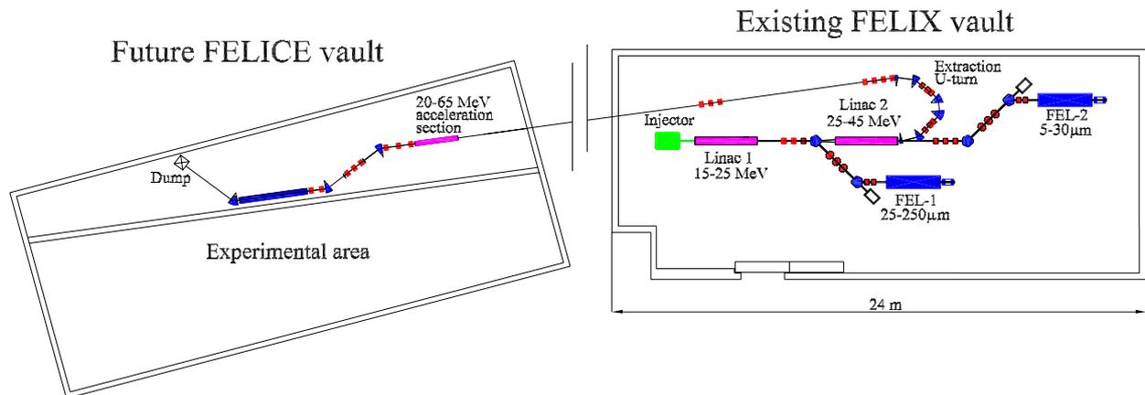
Figure 1: General layout of the FELICE free electron laser facility.
