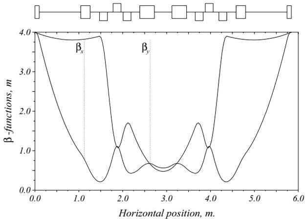
Figure 2: Optical functions in the beam extraction section for the zero chromaticity and chronicity as calculated with the MAD code.
