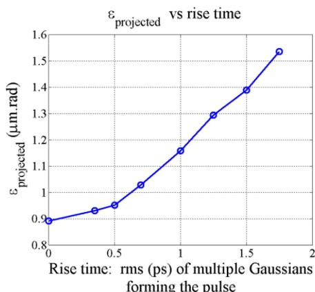
Figure 2- Projected emittance vs rise time (computed for thermal emittance of 0.6mm.mrad)
