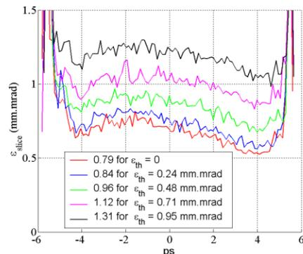
Figure 1. Slice emittance along bunch at the end of beamline for various thermal emittances.
