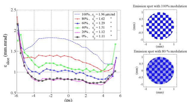
Figure 3- Slice emittance for different modulation of the densities on emission spot;  $r = 1\text{mm}$ ;  $\epsilon_{th} = 0.3\text{ mm.mrad}$ .
