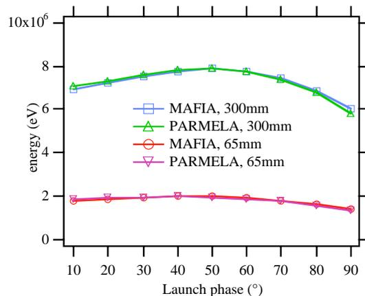
Figure 3. Variation of bunch energy with launch phase, 64 MV/m on cathode, 43 MV/m cells 2 & 3, II- mode.
