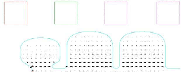
Figure 2. Profile of 3-cell RF gun showing MAFIA calculated electric fields and position of solenoid coils.
