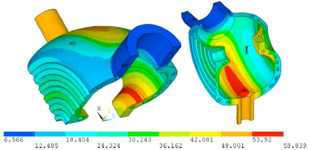
Figure 9. Temperature calculated by ANSYS
