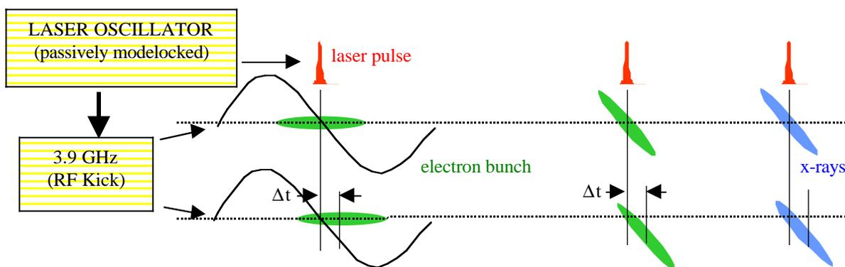
Figure 1. Time-position-angle correlation of deflected bunches
