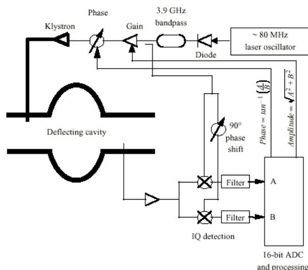
Figure 4. Deflecting cavity feedback systems
