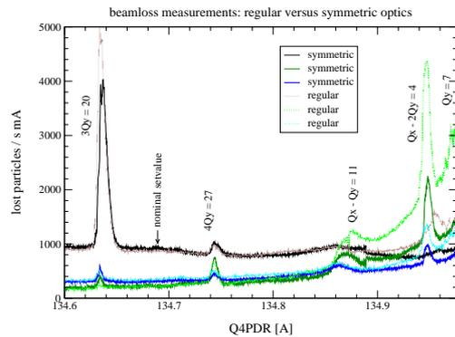
Figure 5: Particle losses for standard (solid line) and symmetry corrected (dotted, lighter colour) optics detected at different ring positions
