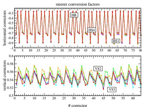
Figure 3: Fitted steerer conversion factors for horizontal (top) and vertical (bottom) correctors
