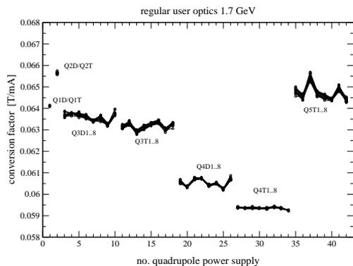
Figure 1: Fitted quadrupole conversion factors for measurements taken during more than two years, sorted by power supply families
