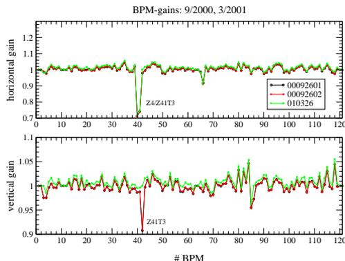
Figure 2: Resulting BPM gains for 3 typical measurements
