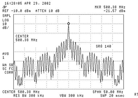
Figure 4: Typical multi-bunch spectrum around 500 MHz. Number of bunches is 400 with 68 ion-clearing gap.
