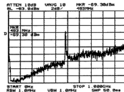
Figure 3: Single-bunch spectrum of IDBPM81 button signal. Note large peak at 483 MHz. Trace was smoothed and averaged.
