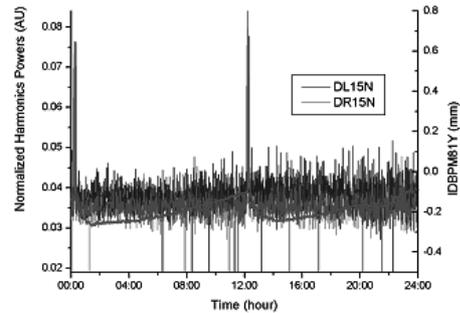
Figure 6: Comparison of time variations of two representative rotation harmonics at 983 MHz (top trace), 1017.2 MHz (middle trace), and IDBPM81 vertical orbit signal (bottom trace). Peaks in IDBPM81Y signal at 0 AM and 1 PM are due to beam injections.
