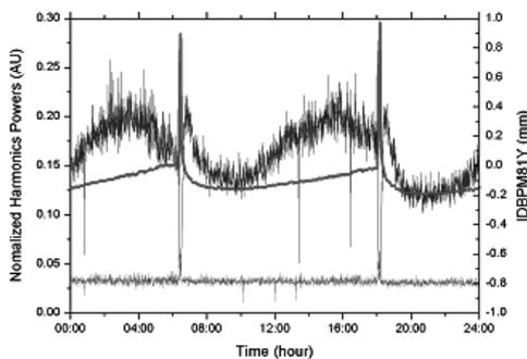
Figure 5: Comparison of time variations of 483 MHz (top trace), IDBPM81 vertical orbit signal (middle trace), and 517.2 MHz (bottom trace). Peaks in IDBPM81Y signal at 9 AM and 9 PM are due to beam injections.
