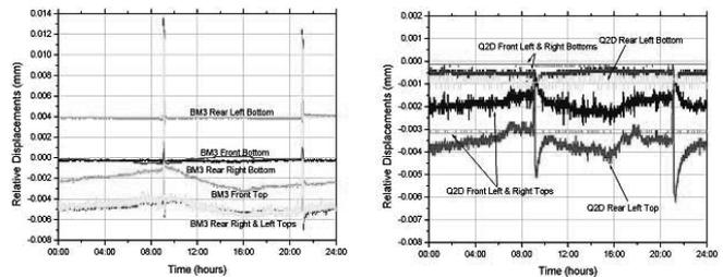
Figure 1: Relative (vertical) displacements of bending (left) and quadrupole (right) magnets at cell#4 during normal machine operation. Spikes around 9 AM and 9 PM are due to beam injection.
