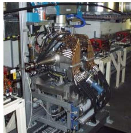
Figure 3: Booster cavity
