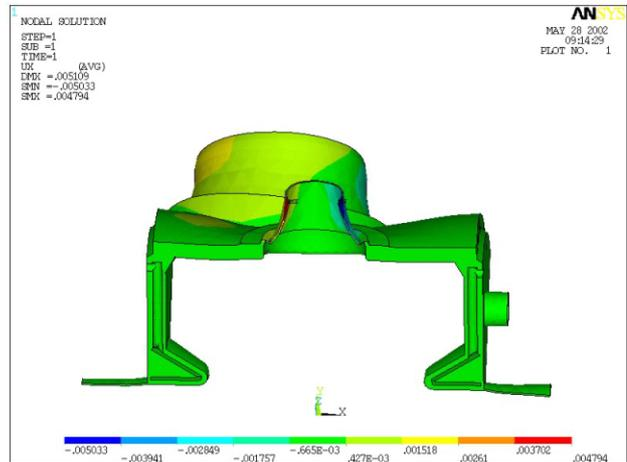
Figure 8: Thermal displacement of nose cones
