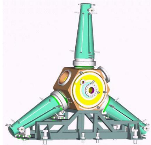
Figure 1: High power HOM damped cavity, with 3 CWCT's and test support
