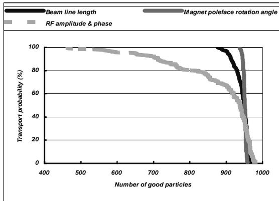
Figure 2. Beam transport probability with respect to various types of error
