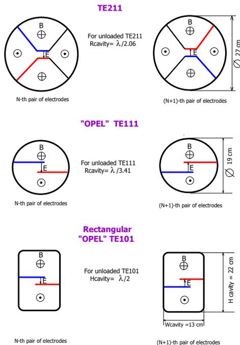
Figure 1: 352.2 MHz funneling structures
