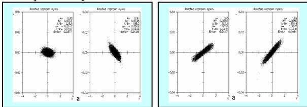
Figure 4: The phase portraits of beam in horizontal and vertical planes on the entrance and exit of funnelling at energy 5 MeV.
