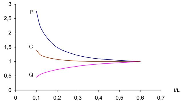
Figure 10: RF losses, Capacity, Q-factor vs  $l/L$
