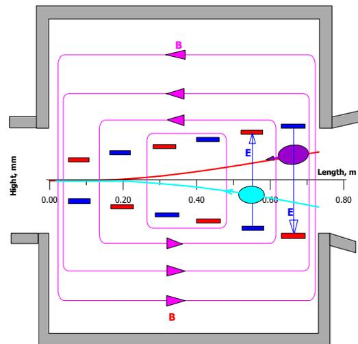
Figure 3: Resonance merging of two beams
