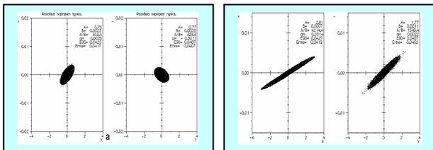
Figure 5: The phase portraits of beam in horizontal and vertical planes on the entrance and exit of funnelling at energy 25 MeV.
