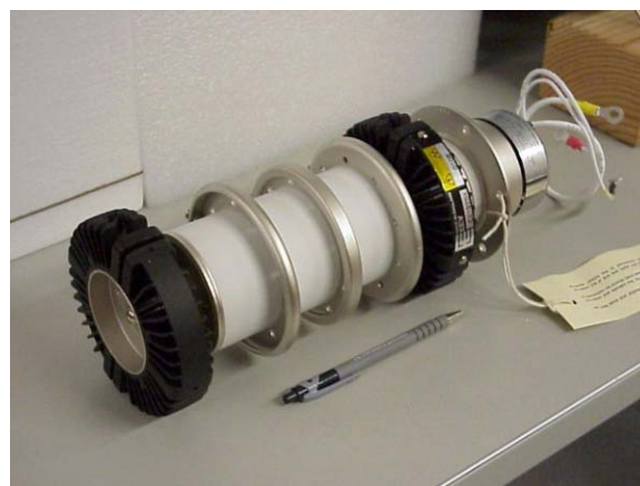
Figure 3: CX1925X thyatron picture.
