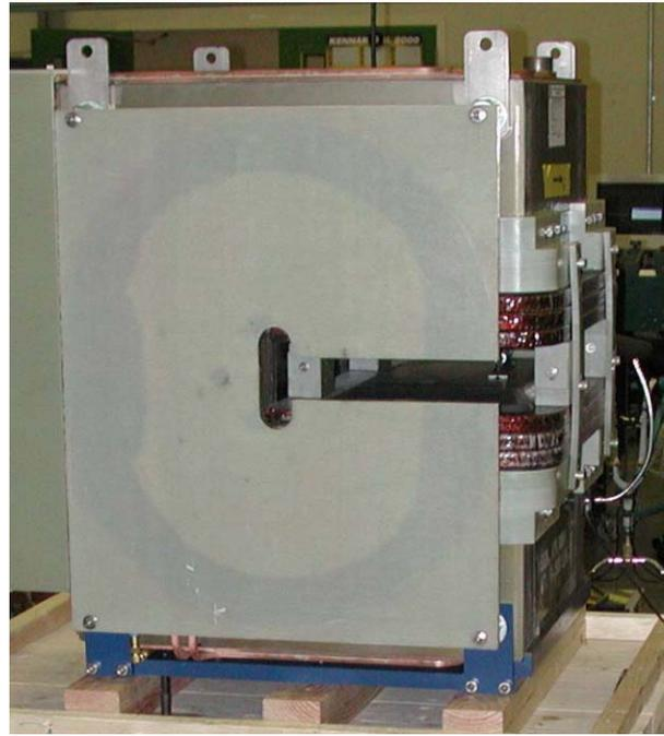
Fig. 1. Photograph of the finished IPF kicker magnet shortly after delivery to Los Alamos.
