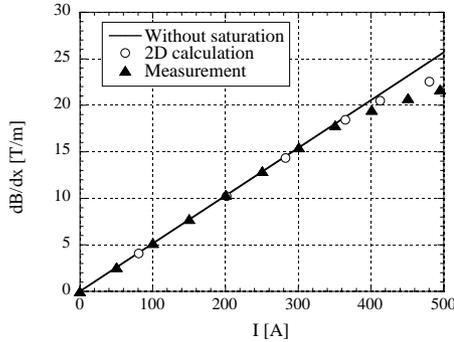
Figure 2: Excitation curve of the quadrupole prototype.
