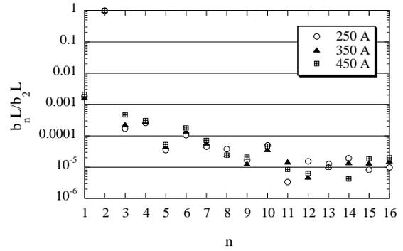
Figure 5: Multipole field amplitudes normalized by the quadrupole component.
