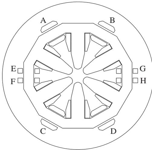
Figure 8: Configuration of the auxiliary coils on SF.
