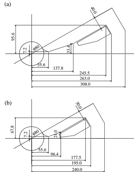
Figure 6: Geometry of the sextupoles (a) SF and (b) SD.
