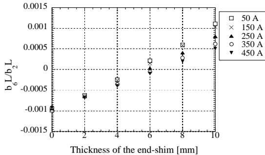
Figure 4: Dependence of the dodecapole to quadrupole ratio on thickness of the end-shimming.
