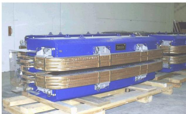
Figure 1: One of the completed CLS dipole magnets.
