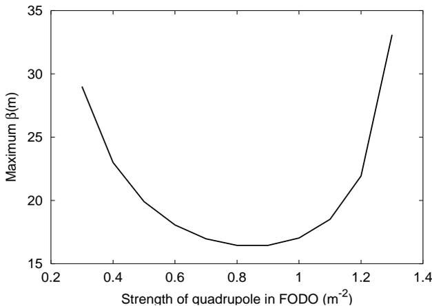
Figure 2:  $\beta_{max}$  as a function of FODO quadrupole strength
