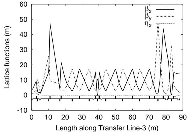
Figure 3: Lattice functions in TL-3
