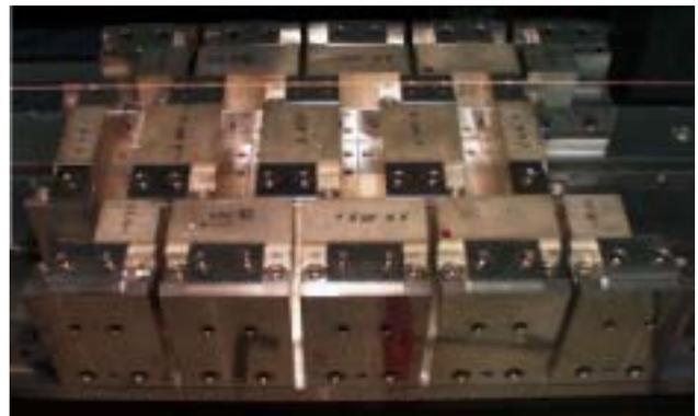
Figure 7: Two-period prototype undergoing magnetic measurements
