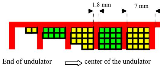
Fig. 2 For a period length of 14 mm and a  $k$ -value close to 2 each groove is filled with 16 wires. Towards the end of the undulator the number of the wires is reduced. The cross-section of one wire is about  $1 \text{ mm}^2$ . Wires with the same color (or grey values) have identical current directions.
