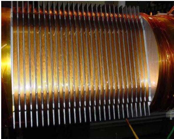
Fig. 3 Photo of the undulator showing the section close to the beam (see fig. 1). The dimensions are defined in fig. 2
