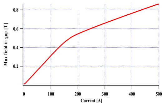
Fig. 6 The measured influence of the saturation of the iron on the maximum magnetic field.
