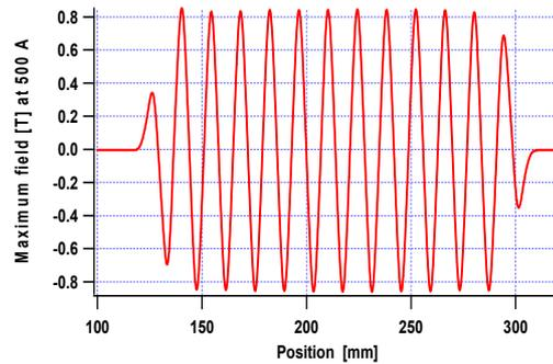
Fig. 5 Measured field along the trajectory with a current of 500 A (almost identical with  $500 \text{ A/mm}^2$ ). The gap is 5 mm.
