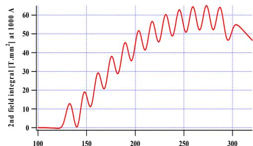
Fig. 8 The measured 2<sup>nd</sup> field integral at a current of 1000 A/mm<sup>2</sup>
