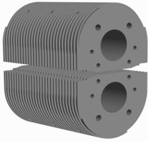
Fig. 1 The iron body of the undulator with the grooves for the superconductive wire. The beam travels along the gap. Through the big holes in the lower and upper part flows LHe
