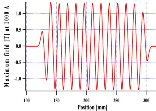
Fig. 4 Measured field along the trajectory with a current of 1000 A (almost identical with  $1000 \text{ A/mm}^2$ ). The gap is 5 mm.
