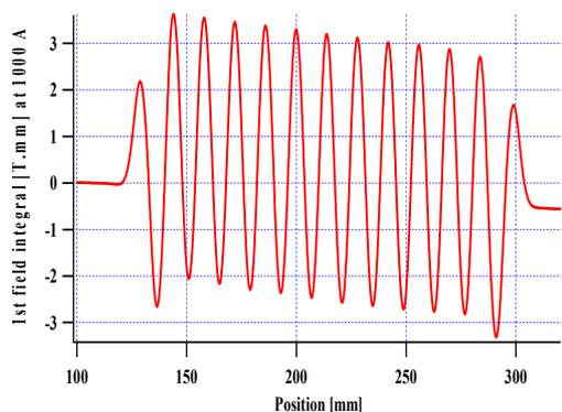
Fig. 7 The measured 1st field integral at a current of 1000 A/mm<sup>2</sup>. The residual error is about -0.6 T.mm
