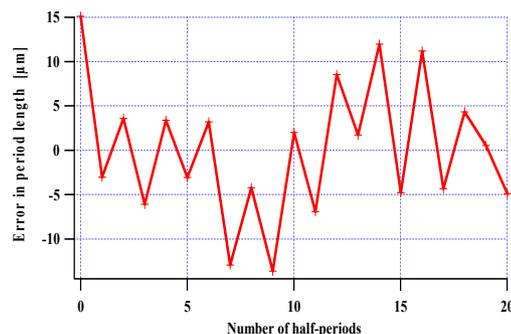
Fig.9 Measured deviation of the half-period length from the value of 7 mm. The specification asked for a maximum deviation of 20 µm, the measured value is significantly smaller.
