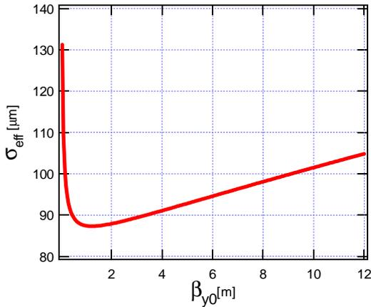
Figure 1: Effective source size as a function of the vertical beta function at the centre of undulator.
