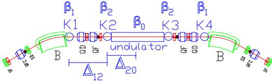
Figure 3: Lay-out of one superperiod of the LNLS storage ring. The fast kicker positions are indicated by circles.
