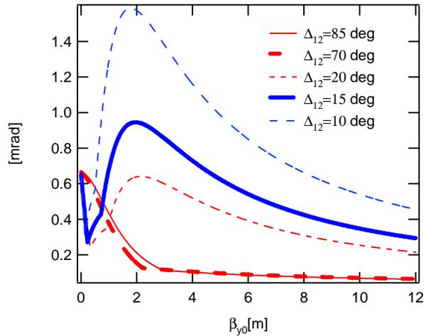
Figure 4: Maximum kicker strength per mm orbit displacement as a function of the vertical beta function at the centre of the straight section for various values of the betatron phase advance between the first two kickers.
