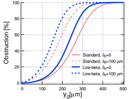
Figure 2: Obstructed fraction of light intensity as a function of pulsed beam displacement for different machine optics and different initial DC displacement  $\delta_0$ .
