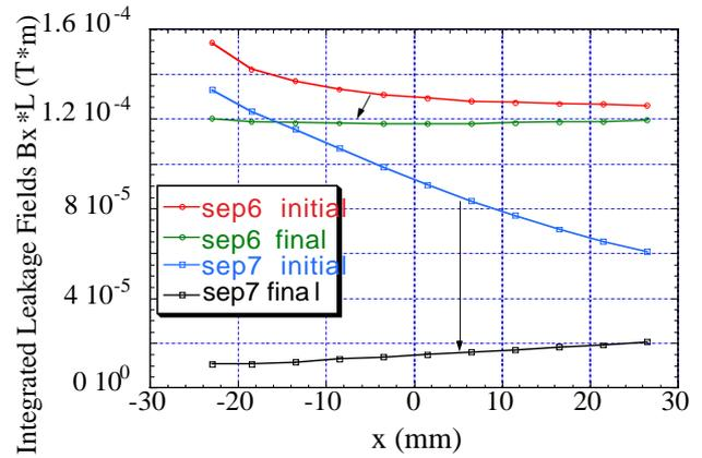
Figure 5: Horizontal component of integrated leakage fields. The central orbit is  $x = 0$  and the bump orbit is  $x = -14.5$ .
