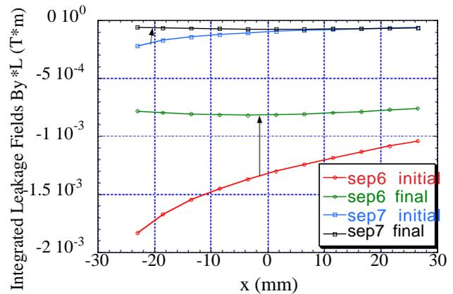
Figure 6: Vertical component of integrated leakage fields.
