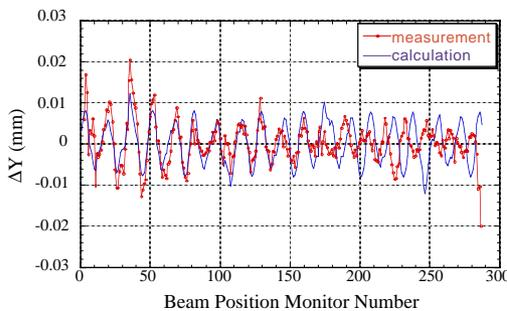
Figure 8: Measured and calculated cod for vertical direction.
