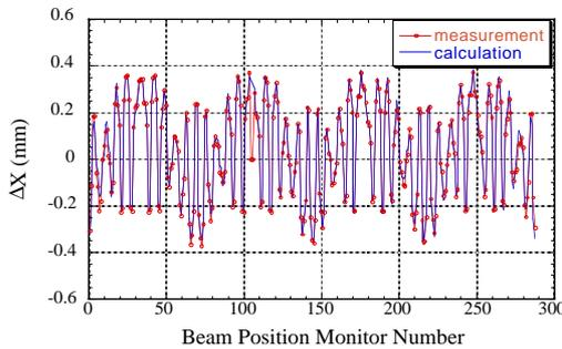
Figure 7: Measured and calculated cod for horizontal direction.
