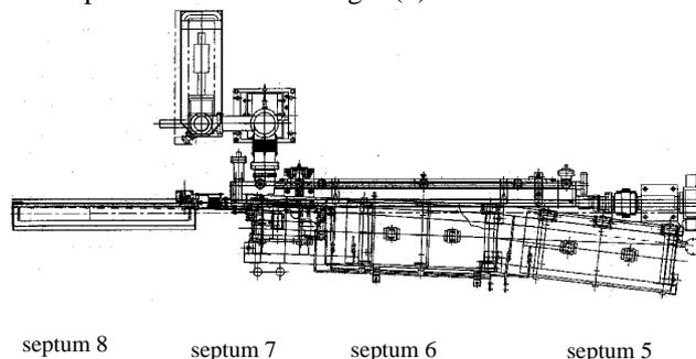
Figure 1: Arrangement of injection magnets.
