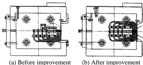
Figure 2: DC septum magnet before and after improvement.
