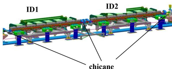
Figure 1: structure of the UE212 twin polarized undulator having two MV power supplies we were able to implement quasi-periodic mode.
