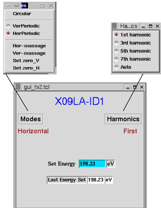
Figure 3: Tcl/Tk GUI for the UE212
