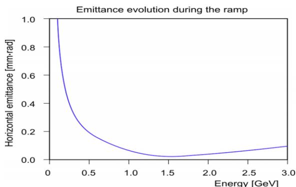
Figure 5. Beam emittance during the energy ramp.
