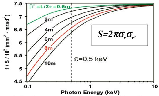
Figure 3. Brightness vs photon energy and local beta.
