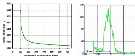
Figure 6. Number of transmitted particles (left) and longitudinal distribution in the 3GHz linac (right).
