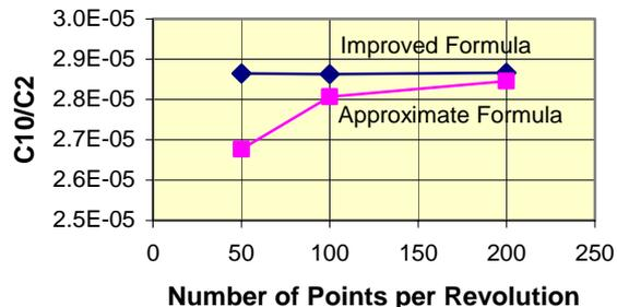
Fig. 3 Integrated 20<sup>th</sup> pole vs. sampling points from two formulas.
