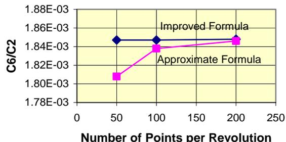
Fig. 2 Integrated dodecapole vs. sampling points from two formulas.
