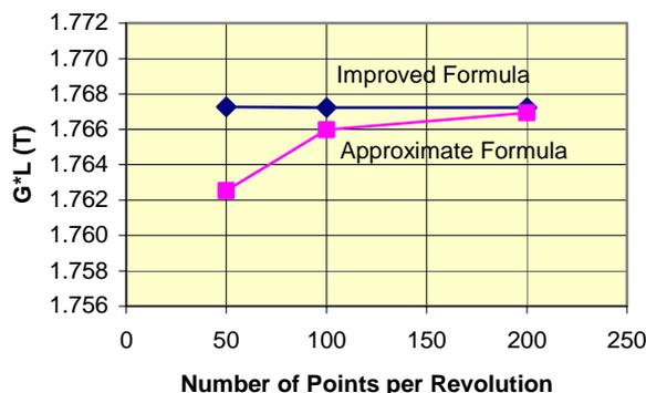
Fig. 1. Integrated gradient vs. sampling points from two formulas.
