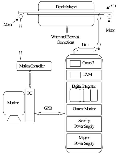
Fig. 5 Experimental setup.
