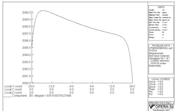
Fig. 2 Field distribution along the x-axis at y=z=0.
