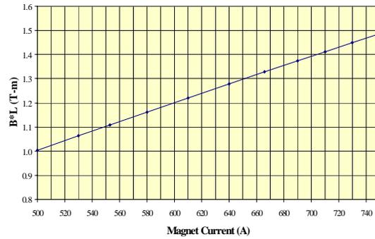
Fig. 8 Integrated fields vs. current.
