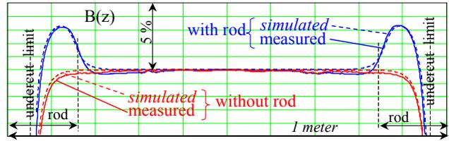
Figure 5. B field simulation/measurement in the cavity with flush tuners, with/without dipolar rod stabilizers.
