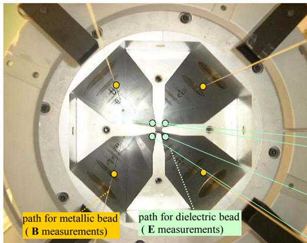
Figure 1. Electric and magnetic bead-pull measurements.
