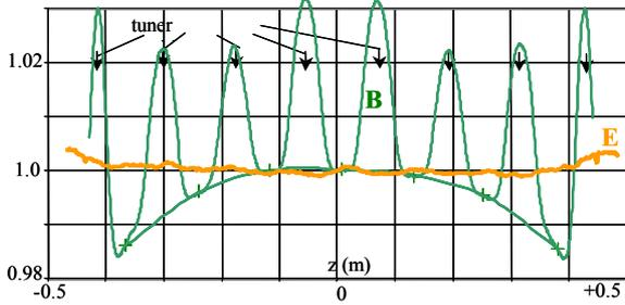
Figure 3. Field measurements in the tuned cold model from E-field perturbation. B exhibits a slight curvature.
