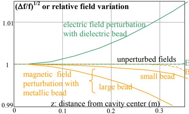
Figure 4. Simulation of bead-pull measurements.
