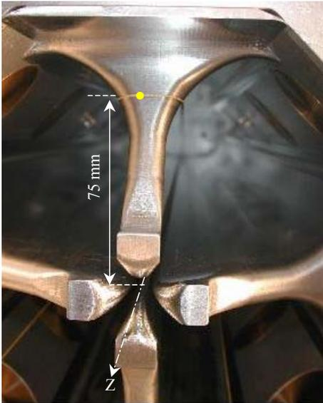
Figure 7. Bead-pull  $B^2$  measurement in undercut region.
