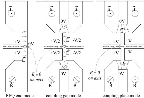
Figure 6. Different types of monopolar local modes.
