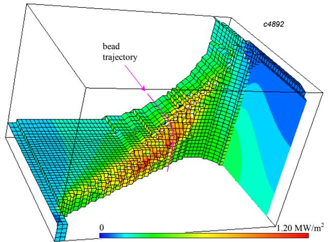
Figure 8. RF losses in undercut computed by MAFIA.
