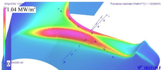
Figure 9. RF losses computed by SOPRANO.
