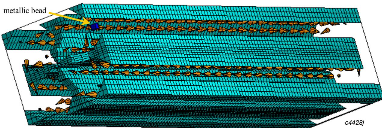
Figure 2. Simulation of magnetic field bead-pull measurement in a 1-m RFQ.
