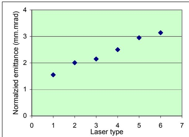
Figure 4: Emittance as a function of laser’s non-uniformity. The laser types correspond to increasing attenuation (see text).
