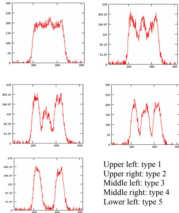
Figure 1: Uniform and non-uniform laser transverse profiles (horizontal axis scale is in pixels)
