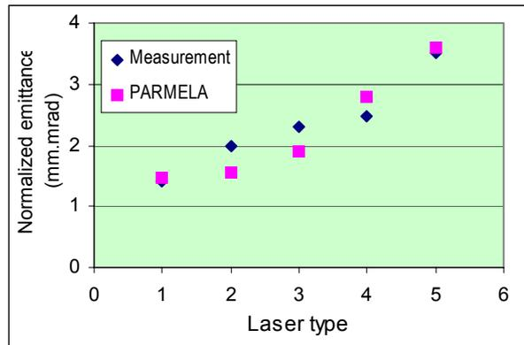
Figure 2: Emittances vs. laser distribution types, arranged by increasing non-uniformity (see text). Type 1 is the unperturbed (most uniform) distribution.
