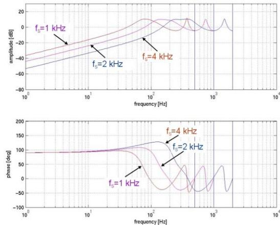
Figure 3: Dependency of closed position feedback loop on the BPM sampling rate  $f_s = 1$  kHz, 2 kHz and 4 kHz.
