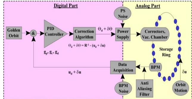
Figure 2: Block diagram of global orbit feedback.
