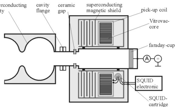
**Figure 5: Schematic Design of the CHECHIA CCC**
