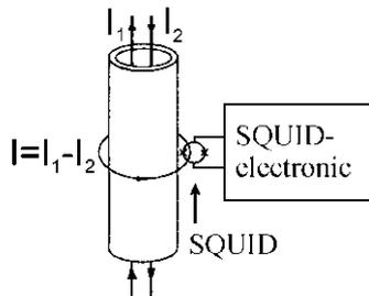
**Figure 1: Principle of a Current Comparator**
