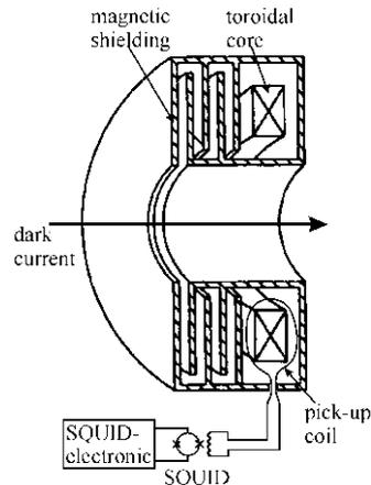
**Figure 2: Schematic view of magnetic shielding, pickup coil and SQUID**
