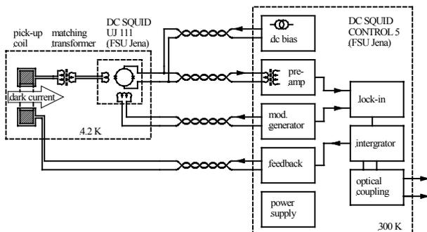
**Figure 4: Cryogenic Current Comparator (simplified scheme)**
