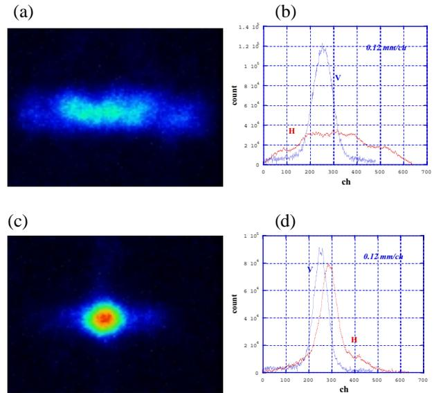
Figure 7: Electron cooling experiment in fixed energy of 6 MeV/u. Beam profiles of : (a)(b) before cooling, (c)(d) after 2.1 sec cooling.
