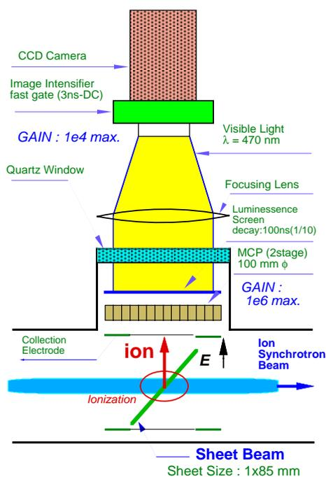
Figure 2: Layout of the beam profile detector.
