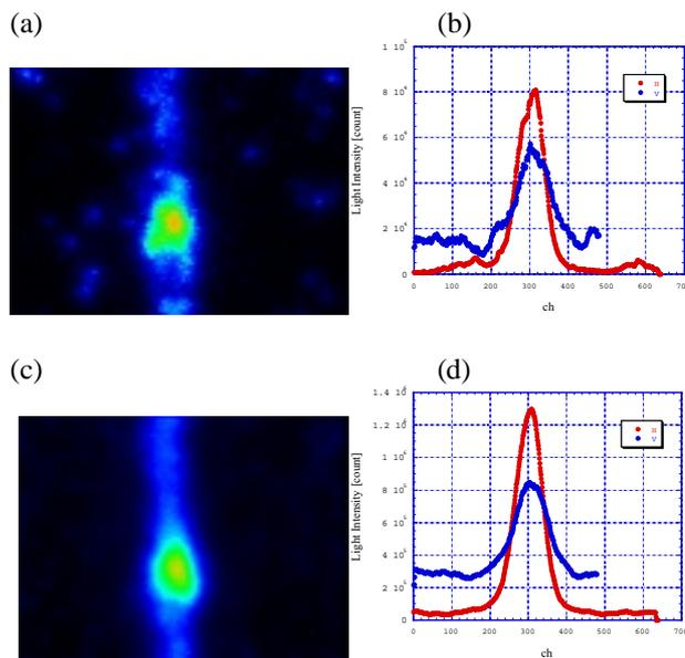
Figure 4: (a)(b) One shot beam profile of 5  $\mu$ A proton beam with camera gate of 20  $\mu$ sec, (c)(d) 20 cycles accumulated one with the same conditions.
