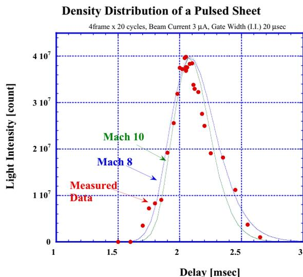
Figure 3: Time dependence of the density distribution of a 120  $\mu$ sec pulsed oxygen sheet beam.
