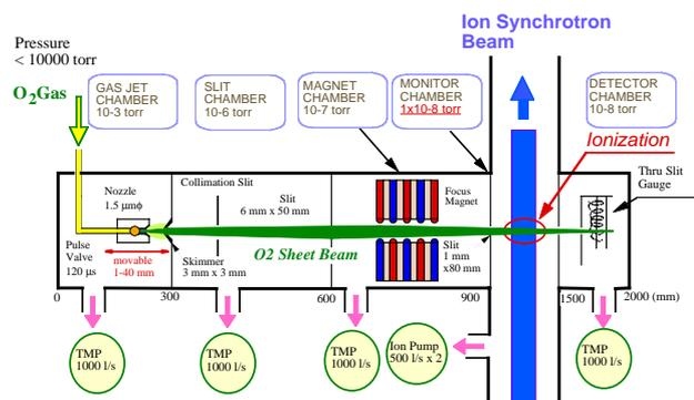
Figure 1: Schematic view of the gas sheet beam profile monitor.
