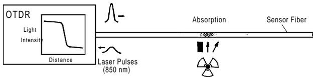
Figure 3: Basic principle of the OTDR measurement [1].
