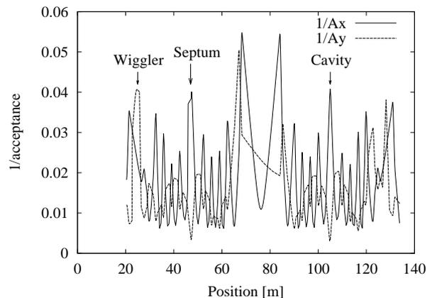
Figure2: Inverse of DELTA acceptance starting from the wiggler (20 m) counter clockwise around DELTA. The maxima of the horizontal and vertical curves show the minimum acceptances at DELTA.
