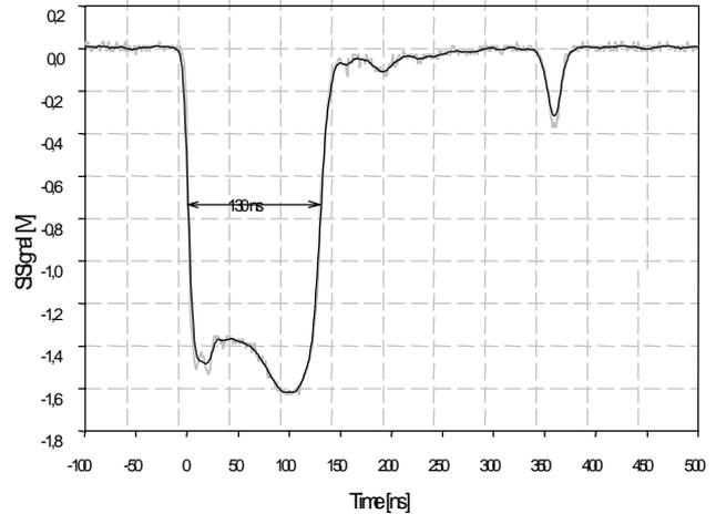
Figure 6: Beam loss in BoDo after injection of a 130 ns long linac pulse. Revolution time of BoDo is 168 ns.
