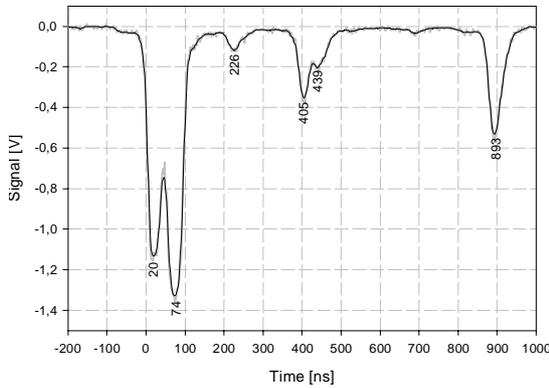
Figure 5: Cerenkov light signal from the photomultiplier. Three turns in DELTA (one turn = 384 ns). Several peaks per turn result from different centres of beam loss.
