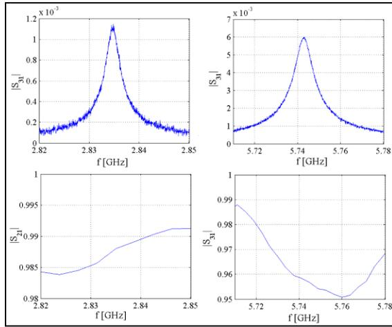
Figure 4: measured transmission coefficients ( $S_{21}$ ,  $S_{31}$ ).
