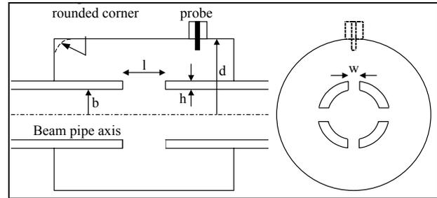
Figure 1: sketch of the bunch length monitor.
