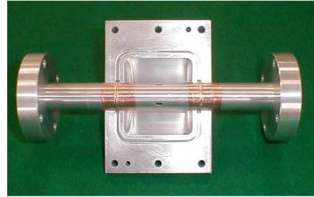
Figure 3: bunch length monitor prototype.
