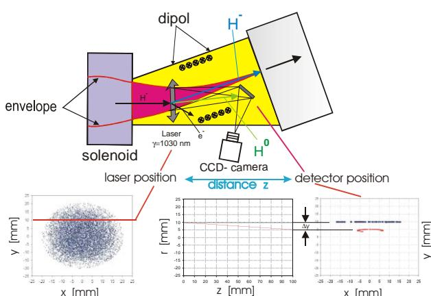
Figure 5: Measurement principle and the diagnostic set up of the laser driven emittance measurement device.
