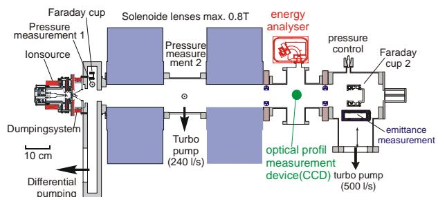
Figure 4: Schematic drawing of the LEBT section with diagnostics in a first testing phase.
