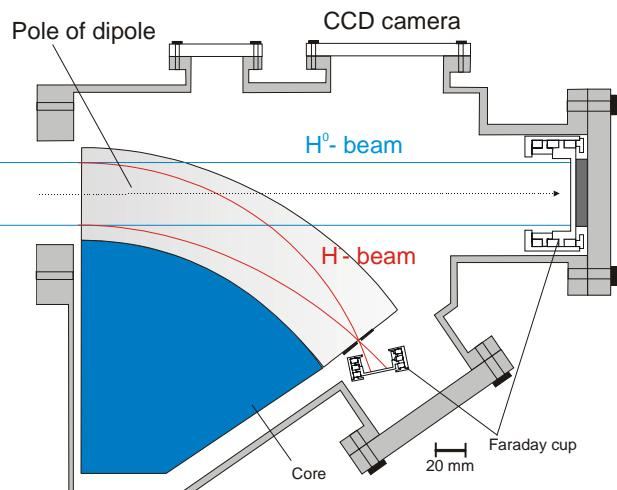
Figure 2: Scheme of the diagnostic chamber and dipole. The separation of neutralized H-atoms from the ion beam is plotted.
