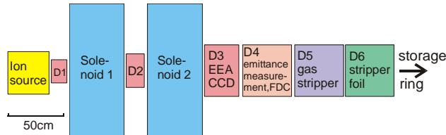
Figure 1: LEBT section with four diagnostic chambers (D1-D4) to investigate the beam transport properties and two diagnostic chambers to investigate the gas cell (D5) and the stripping at a stripper foil (D6).
