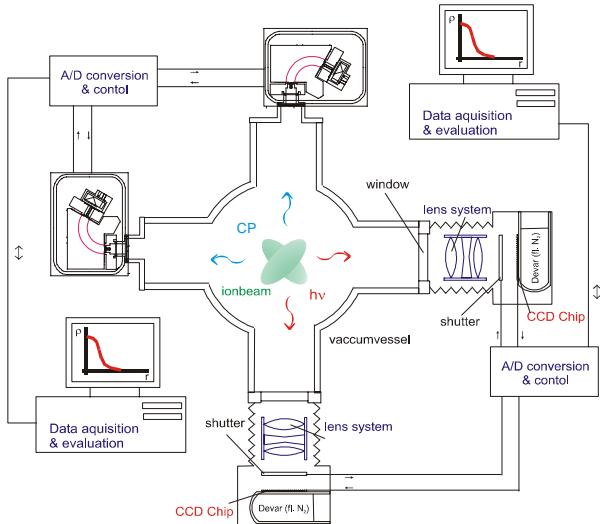
Figure 3: Diagnostic set up of two CCD-cameras and two spectrometers in orthogonal arrangement.
