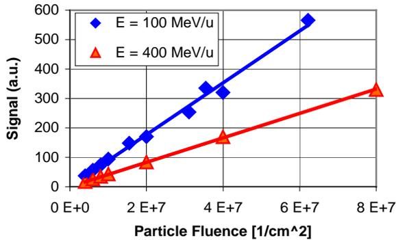
Figure 5: Viewing Screen characteristic line for carbon beams; lens aperture for all measurements fixed to 5.6
