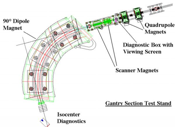
Figure 3: Equipment of the gantry section test stand (schematic view)
