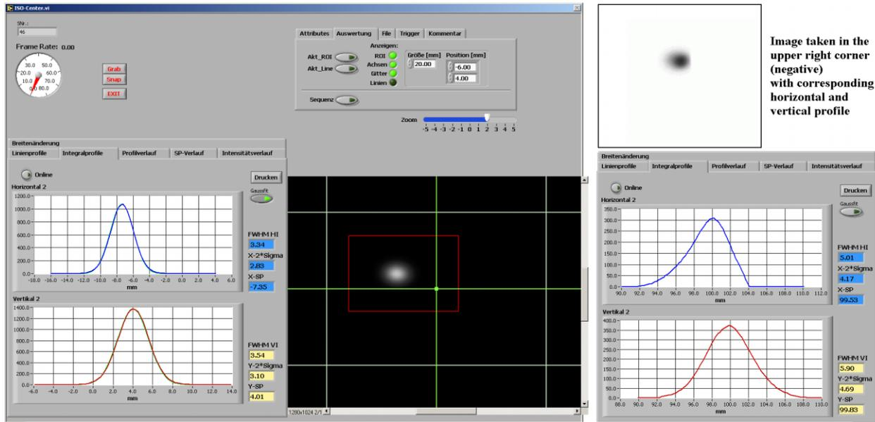
Figure 4: Screenshot of the data acquisition and online analysis programme (left) – beam spot and profiles measured near the centre of the screen. A second image (right side with accompanying profiles) taken with both scanner magnets excited to 90% of the maximum field.
