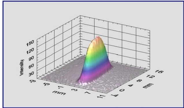
Figure 1: Intensity plot of a 356 MeV/u <sup>12</sup>C<sup>6+</sup>-beam on a P43 target
