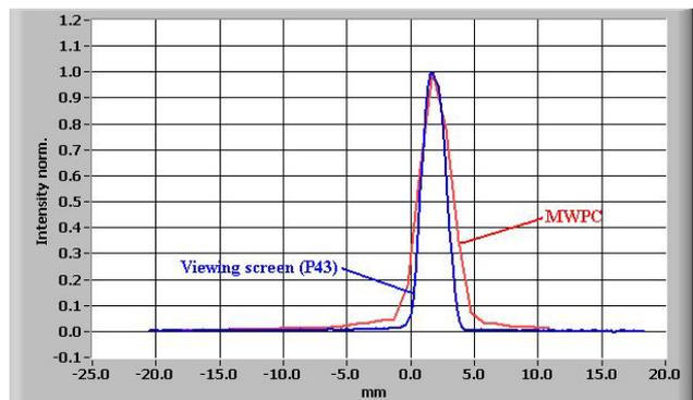
Figure 2: Horizontal profile of a 356 MeV/u <sup>12</sup>C<sup>6+</sup> -beam on a P43 target in comparison to a MWPC measurement
