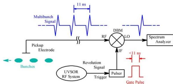
Figure 2: Block diagram of bunch-by-bunch diagnostic system using an electronic analog switch.
