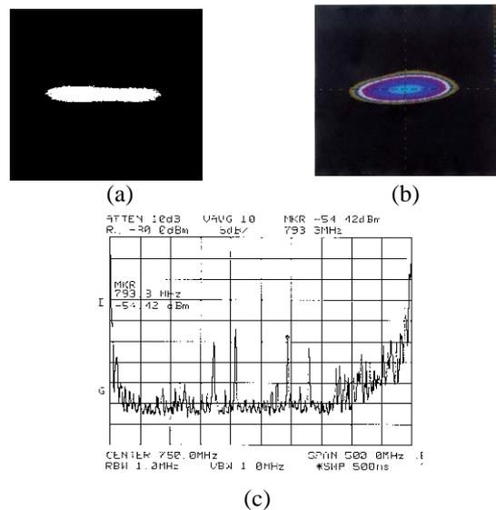
Figure 1: X-ray beam shapes and spectrum when a big longitudinal instability exists.
