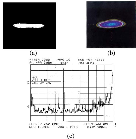
Figure 1: X-ray beam shapes and spectrum when a big longitudinal instability exists.
