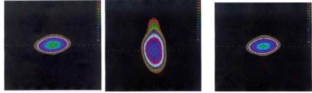
(a) 300mA, SD=138A, SF=92A; (b) 275mA, SD=138A, SF=92A; (c) 275mA, SD=140A, SF=92A
