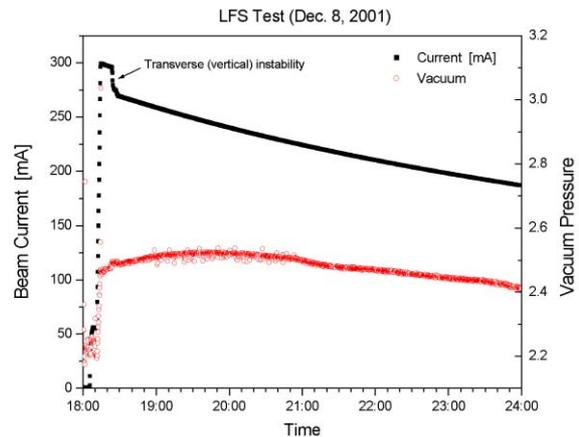
Figure 3: Beam current and vacuum trend when the LFS is working.
