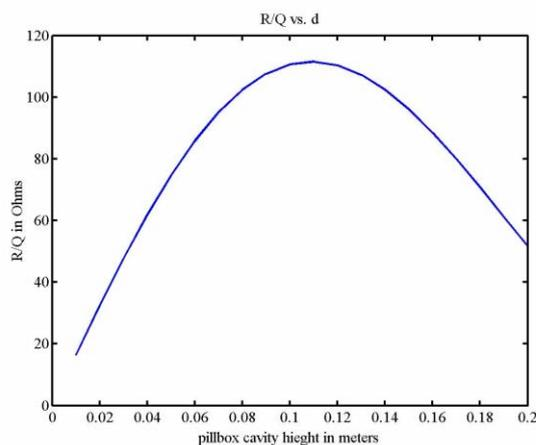
Figure 1: The calculated  $R/Q$  versus cavity height  $d$ .
