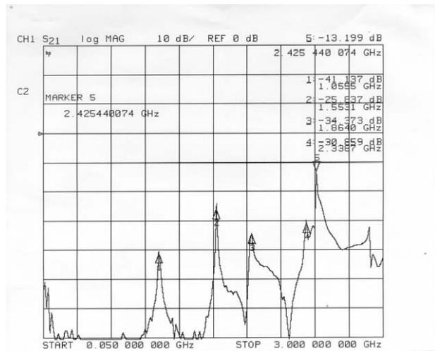
Figure 4: Cavity resonant modes as observed from signal picked up by the coupler
