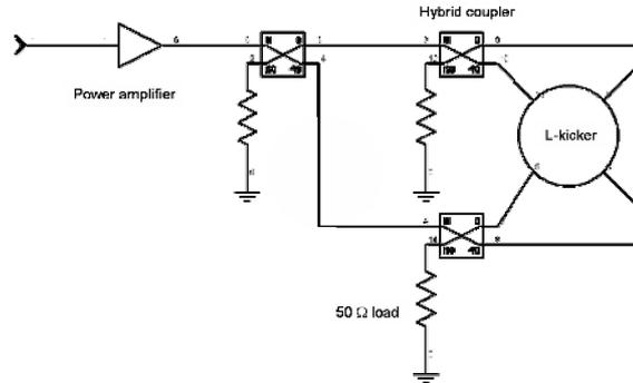
Figure 7: Schematic layout of the rf transmission system for the longitudinal kicker.
