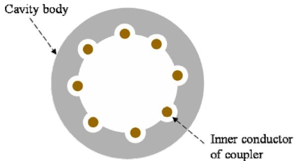
Figure 3: Cross section view of a kicker cavity with eight couplers.
