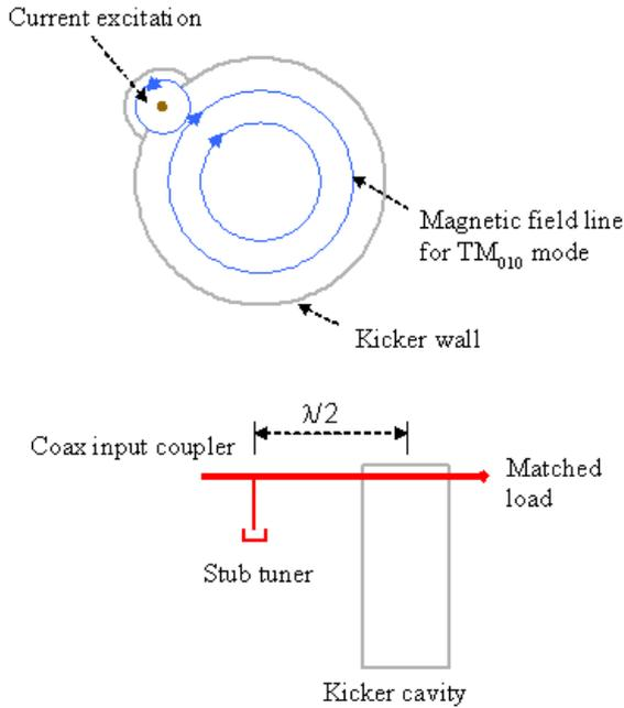
Figure 2: An illustration of the magnetic field coupling scheme for the kicker cavity.
