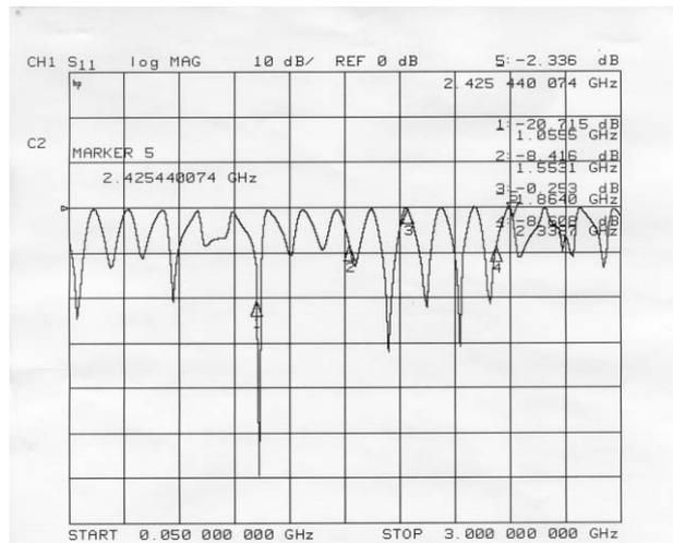
Figure 5: Return loss measured at the one end of the input coupler with properly adjusted matching stub
