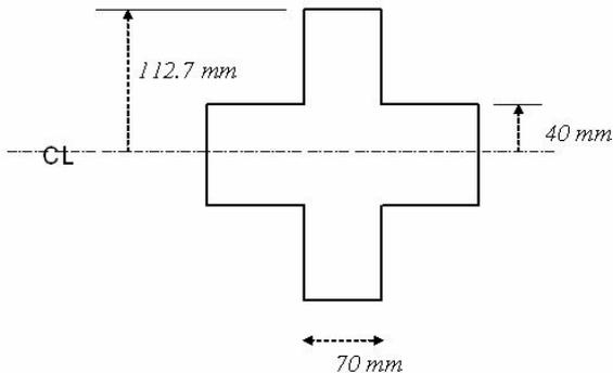
Figure 6: Dimensions of the kicker cavity for preliminary calculations
