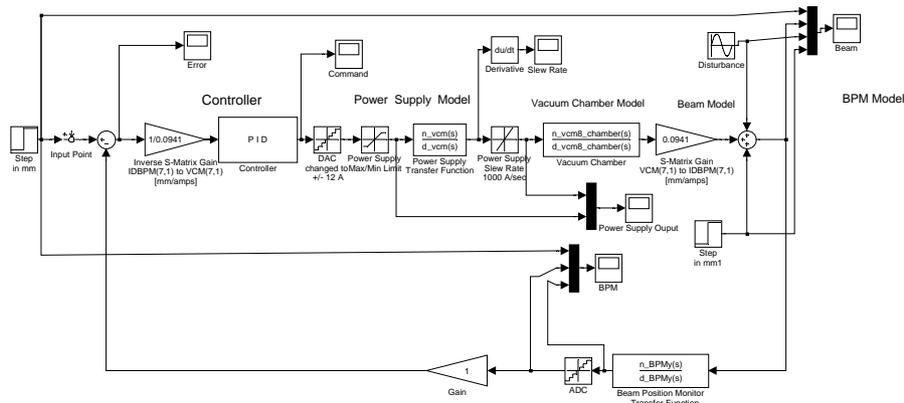
Figure 2: One of the Matlab-Simulink models used to optimize the performance of the smallest building block of the feedback system: One BPM, one ADC and DAC, the controller and one corrector magnet.
