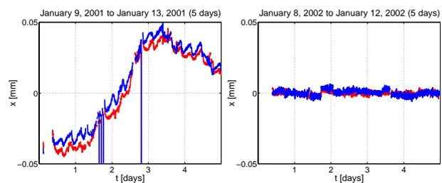
Figure 1: Orbit drift over 5 days in one arc of the ALS with or without rf-frequency feedback.
