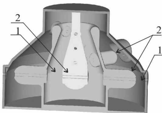
Fig. 2 Accelerator cross-section on fourth beam passage
