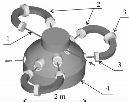
Fig. 1 Schematic view of accelerator complex. 1 – beam path, 2 – bending magnet, 3 – lenses/diagnostics, 4 – cavity.
