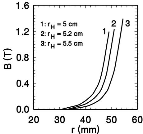
Figure 7: Magnetic field  $B$  inside hexapole of  $B_{max} = 1.4$  T for  $H = 2.8$  cm. Here,  $r_H$ ,  $H$  and  $r$  are inner radius, thickness and cylindrical coordinate of hexapole, respectively.
