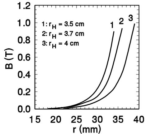
Figure 5: Magnetic field B inside hexapole of  $B_{max} = 0.99$  T for  $H = 2.8$  cm. Here,  $r_H$ , H and r are inner radius, thickness and cylindrical coordinate of hexapole, respectively.
