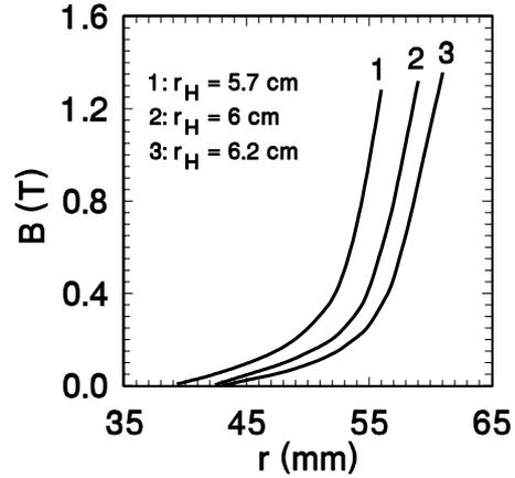
Figure 8: Magnetic field  $B$  inside hexapole of  $B_{max} = 1.365$  T for  $H = 2.8$  cm. Here,  $r_H$ ,  $H$  and  $r$  are inner radius, thickness and cylindrical coordinate of hexapole, respectively.
