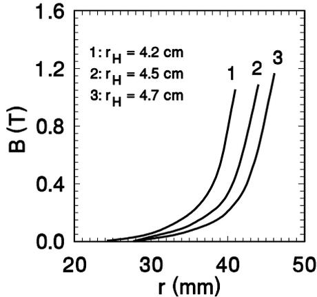
Figure 6: Magnetic field  $B$  inside hexapole of  $B_{max} = 1.17$  T for  $H = 2.8$  cm. Here,  $r_H$ ,  $H$  and  $r$  are inner radius, thickness and cylindrical coordinate of hexapole, respectively.
