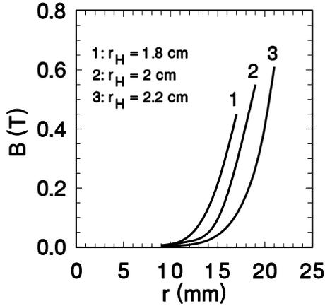
Figure 2: Magnetic field B inside hexapole of  $B_{max} = 0.61$  T for  $H = 2.8$  cm. Here,  $r_H$ , H and r are inner radius, thickness and cylindrical coordinate of hexapole, respectively.
