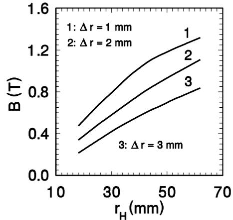
Figure 9: Magnetic field  $B$  inside hexapole as a function of the radius  $r_H$  for different distances  $\Delta r$  from the surface of hexapole  $\Delta r \in \langle 1, 3 \rangle$  mm.
