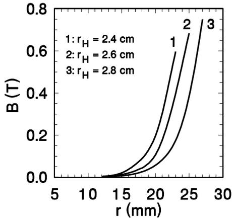
Figure 3: Magnetic field B inside hexapole of  $B_{max} = 0.76$  T for  $H = 2.8$  cm. Here,  $r_H$ , H and r are inner radius, thickness and cylindrical coordinate of hexapole, respectively.
