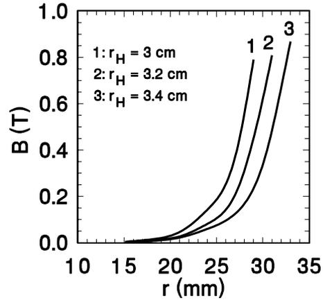
Figure 4: Magnetic field B inside hexapole of  $B_{max} = 0.87$  T for  $H = 2.8$  cm. Here,  $r_H$ , H and r are inner radius, thickness and cylindrical coordinate of hexapole, respectively.
