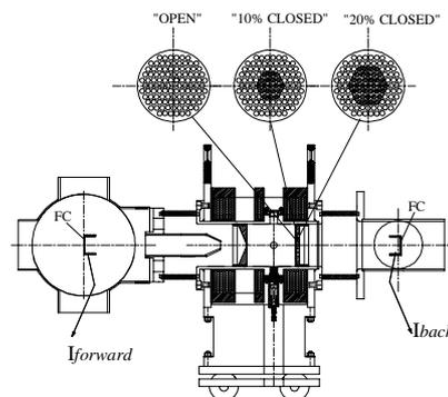
Figure 2: The scheme of experiment on measurement of ion currents from the source.
