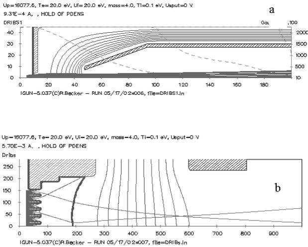
Figure 5: The IGUN simulation of the extraction through the plasma electrode (a), and through the shorting plate (b).
