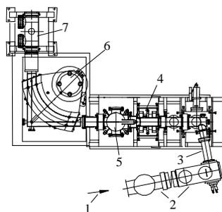
Figure 1: Layout of the DRIBs production station: 1 – primary beam; 2 – target and catcher; 3 – diffusion line; 4 – ECR source; 5 – extraction box; 6 – magnet; 7 – diagnostic box.
