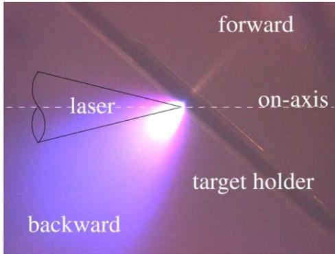
Figure 1: A photograph at the laser irradiation taken from the direction parallel to the laser axis and perpendicular to the  $3\ \mu\text{m}$ -thick Al target foil surface
