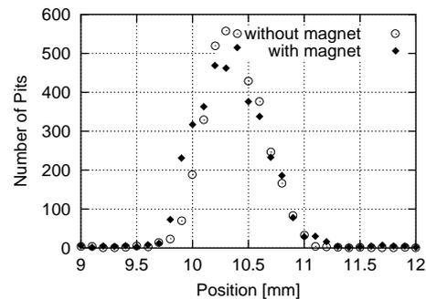
Figure 3: Deflections of etched pits caused by the magnetic energy analyzer (filled diamonds). White circles represent the distribution without magnetic field. Target was Al in  $3\ \mu\text{m}$ -thick.
