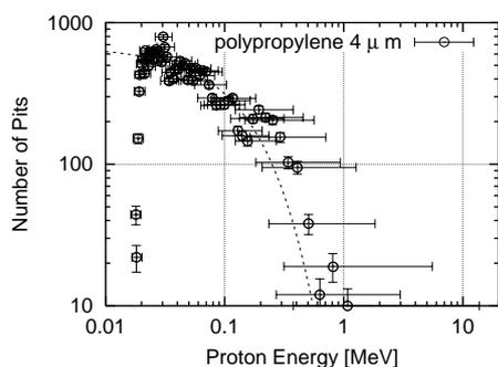
Figure 4: The energy spectrum estimated from the magnetic deflection in backward direction. Target was polypropylene in  $4 \mu\text{m}$ -thick. The reduced curve is  $\sim \exp[-E[\text{MeV}]/0.13]$ .
