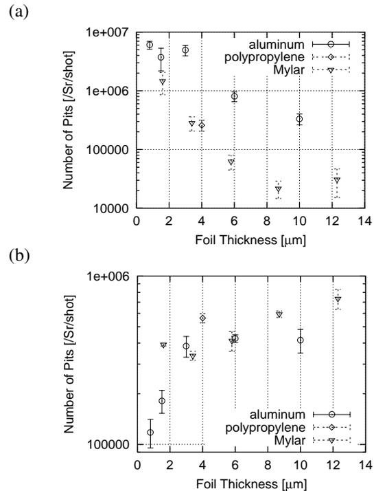
Figure 2: The relation between the number density of etched pits and target thickness. (a): The forward direction. (b): The backward direction.
